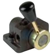
Designed to fit in place of 180908M1(S.42292) interface cover plate which is located on the hydraulic lift cover. Allows the tractors hydraulics to be diverted to external services
